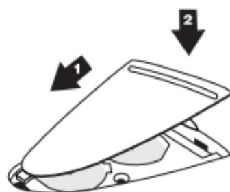
(3) To replace the door, slide it at an angle and push down.
